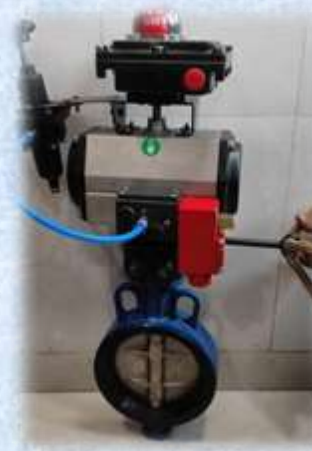
PNEUMATIC ACTUATOR OP. BUTTERFLY VALVE WITH SOV, LIMIT SWITCH, FR & MANUAL OVER RIDE
